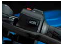
Suzuki Drive Mode Selector (S-DMS)
