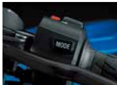
Suzuki Drive Mode Selector (S-DMS)
