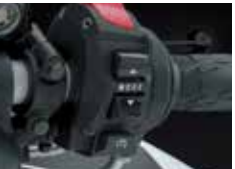
Suzuki Drive Mode Selector (S-DMS)
